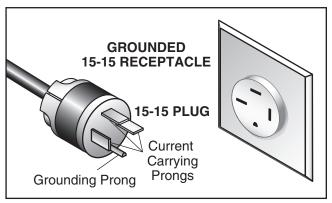
**Figure 1.** Typical 15-15 plug and receptacle.
